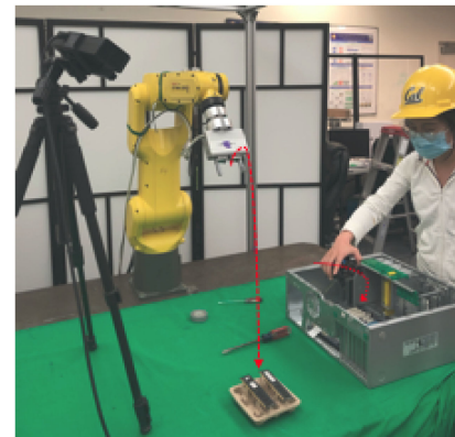
Fig. 7. Robot and human collaborate to assemble a desktop.
