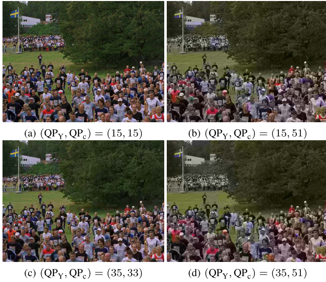
Fig. 3. Exemplar frames encoded using different QP values on luma and chroma. (a) and (c) are encoded without increasing chroma QP values; (b) and (d) are encoded with extreme chroma QP's.
