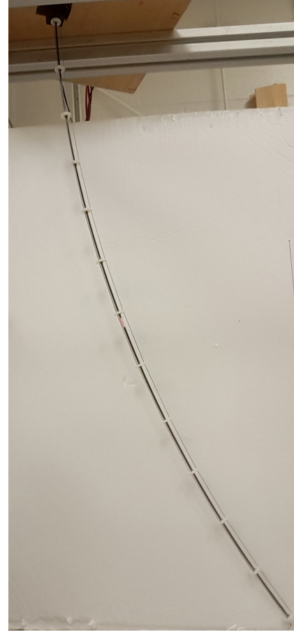
FIGURE 3. THE TENDON-DRIVEN CONTINUUM ROBOT USED FOR EXPERIMENTAL TENSION TESTING.
