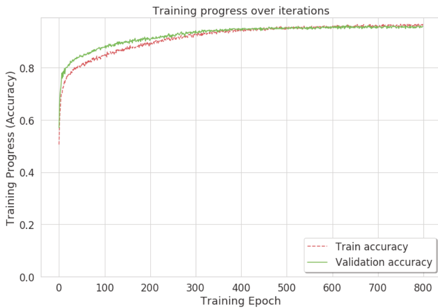
Fig. 11. Training and validation accuracies over iteration of the LSTM 2.
