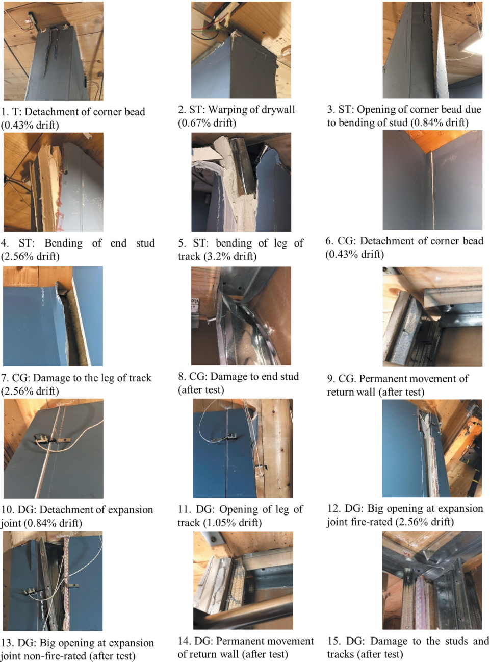
Figure 10. Observed damages to partition walls at various stages of testing: T = Telescoping, ST = Slip-track, CG = Corner gap, DG = Distributed gap.
