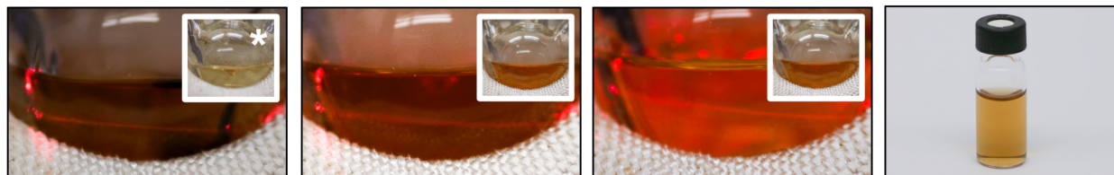
c 300 °C injection: Nanoparticles dissolve and reprecipitate (light scattering disappears then appears)
