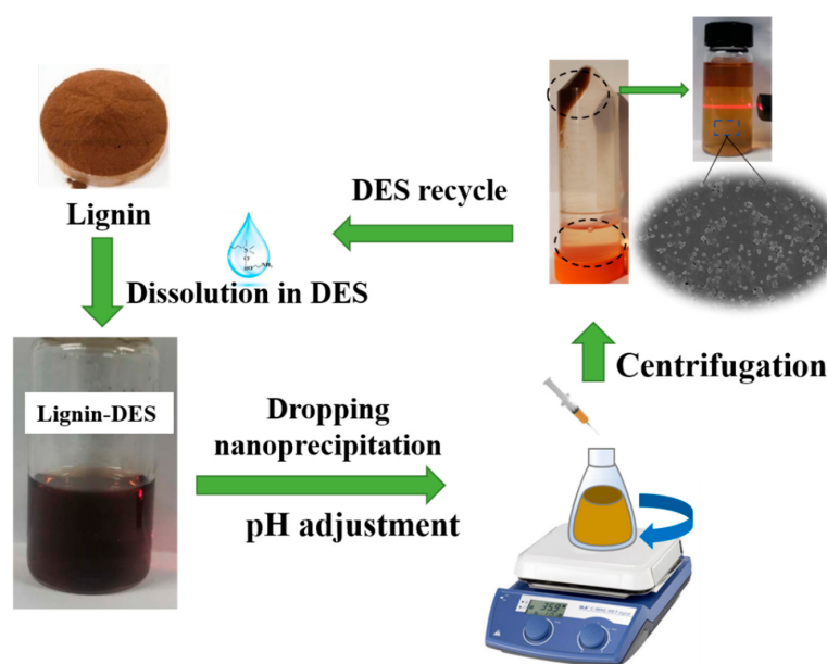
Figure 1. Schematic representation of the preparation procedure of lignin nanoparticles (LNPs). DES: deep eutectic solvent.
