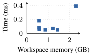
Figure 7: Memory vs. compute for 7 convolution algorithms with 256\times 64\times 56\times 56 input, 3\times 3 kernel, 64 output channels.
