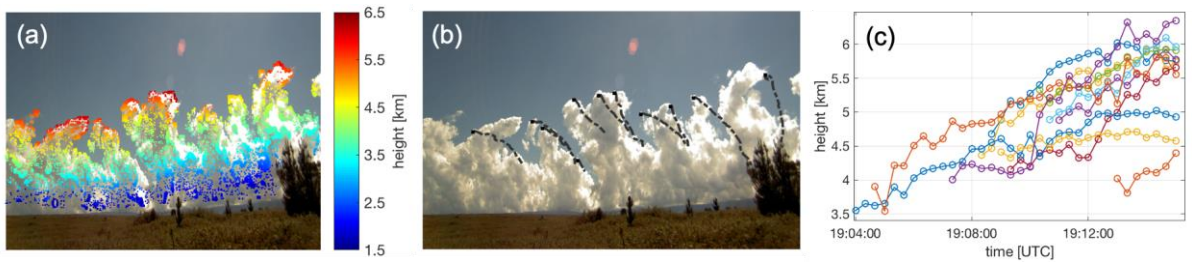
Figure 5. An example of stereo photogrammetric retrieved (a) heights of cloud boundaries, (b) manually tracked growing congestus top tracks, and (c) heights of tracked growing congestus tops in time on 19 December 2018 from 1904 to 1915 UTC.
