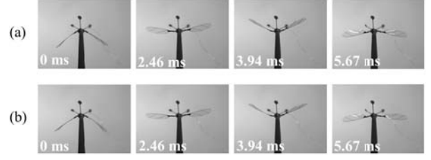
Fig. 6. Wing kinematics are maintained for iso-lift conditions at 140 Hz with a RoboBee operating in typical flight conditions (a) and iso-lift yaw conditions (b).
