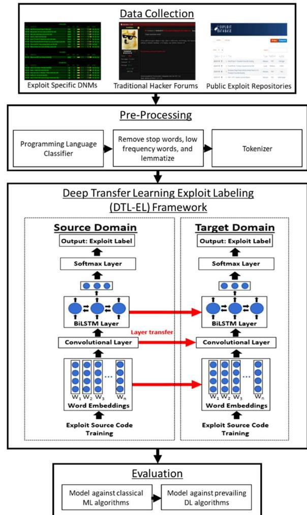
Fig. 3. Proposed Deep Transfer Learning Exploit Labeler Framework
