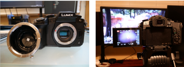
Figure 2: Hardware Setup: On the left, we show our custom lensless camera consisting of a Panasonic Lumix G85 mirrorless camera and diffusion layer attached with a lens mount adapter. On the right is our imaging setup with display monitor for capturing video.
