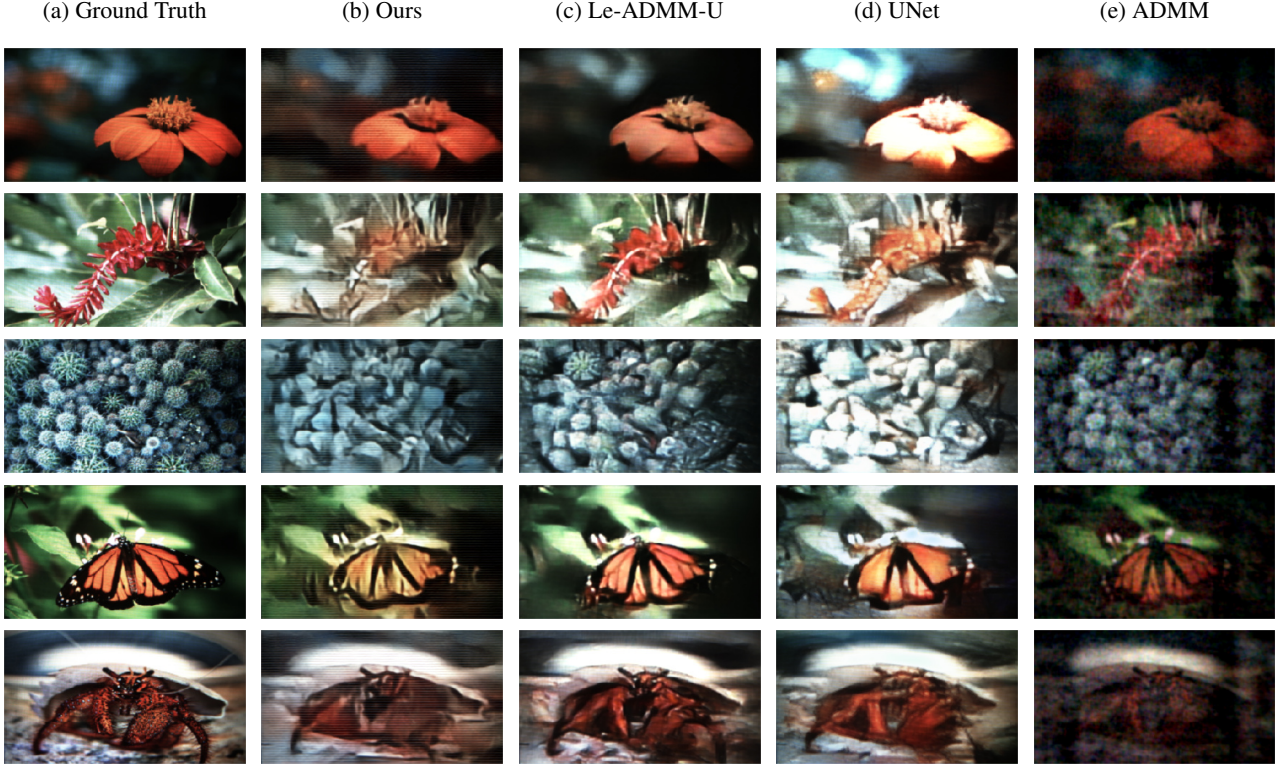
Figure 3: Comparison on DiffuserCam dataset [30]: Reconstruction output of sample images from different models for the DiffuserCam dataset (with the original single PSF). Note that our model performs on-par with the state-of-the-art Le-ADMM-U model.
