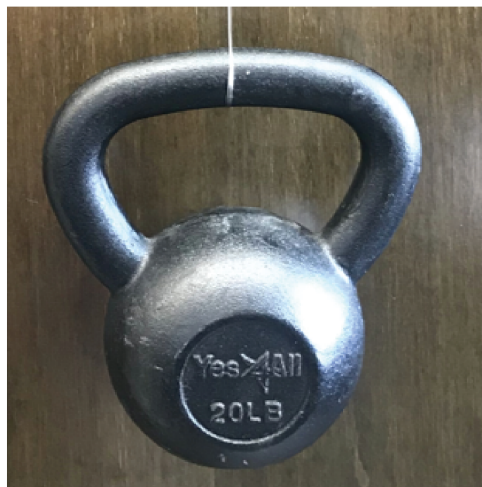
Fig. S21 (a) Left: the adhesive sample prepared for lap shear test. Right: the microscope glass substrate got broken after shear strength reached 2.2 Mpa. (b) Left: adhesive sample is enough to hold 20 pound kettlebell. Right: zoom in photo of 20 pound kettle bell.
