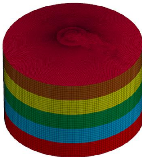
Figure 7. Mesh of silo with aspect ratio H/D = 0.63 and 29,880 shell elements
