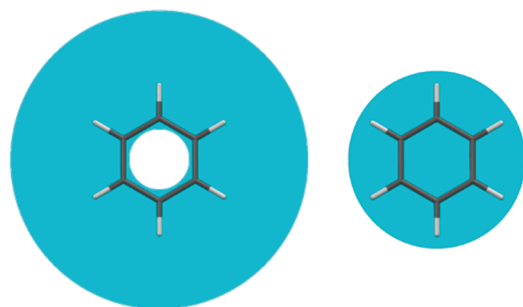
Figure 1. Areas in which attractive interaction energy is larger than -2.0 kcal/mol for benzene–benzene (left) and benzene–cyclohexane (right).
