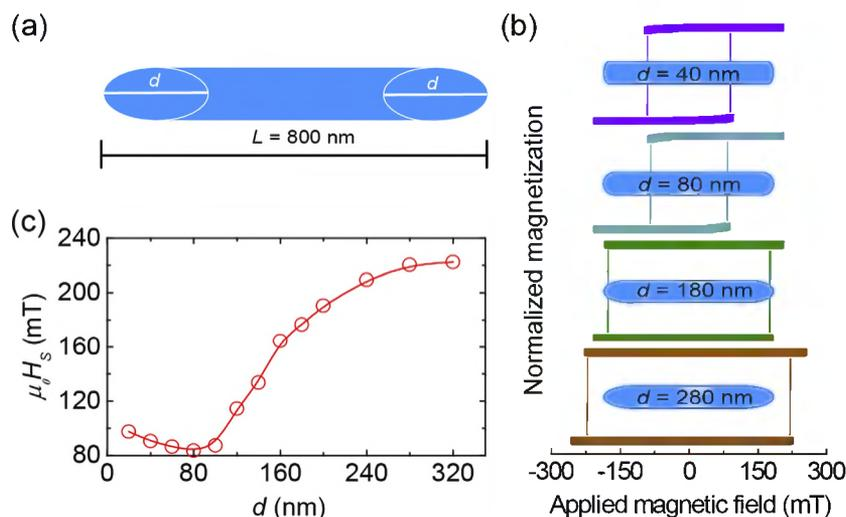
**FIG. 2.** Tuning magnetization reversal with symmetric end-geometries. (a) Schematic of a bar nanomagnet with semi-elliptical ends. The length and width of the bar are 800 and 80 nm, respectively. The elliptical axis length  $d$  is the parameter for tuning the end-geometry. (b) Hysteresis loops of the bar magnets with various identical elliptical axis lengths at the two ends. (c) End shape (or axis length of the semi-ellipse) dependence of the switching fields.
