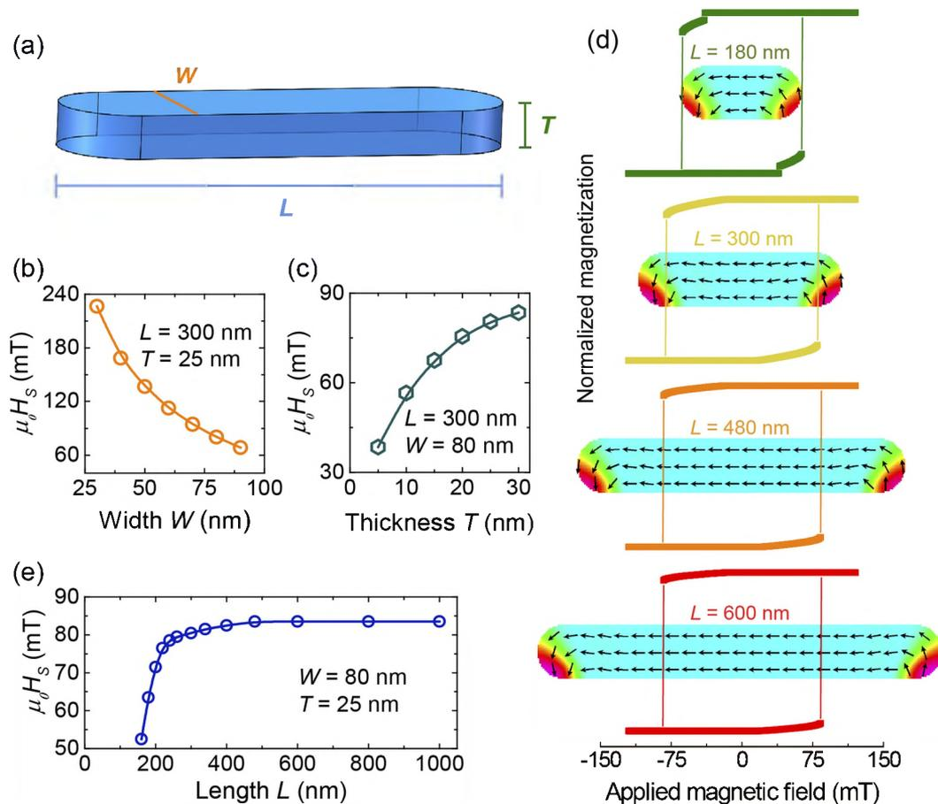
**FIG. 1.** Dimension dependence of magnetization reversal of a bar nanomagnet. (a) Schematic of a nanoscale bar magnet. (b) and (c) The reversal switching field  $H_s$  of the bar magnet as a function of width (b) and thickness (c), respectively. (d) Hysteresis loops of the bar magnets of various lengths. (e) Length dependence of the switching field for a nanomagnet with fixed width,  $W$ , and thickness,  $T$ , as shown in (a).
