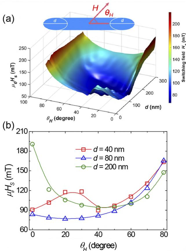
**FIG. 4.** Effects of magnetic field orientation on the magnetization reversal of a bar magnet. (a) Switching field as a function of field orientation  $\theta$  and axis length  $d$  of the semi-ellipses at the symmetric bar ends. (b) Field orientation dependence of the switching field at several selected axis lengths  $d$  of the semi-ellipses at the bar ends.
