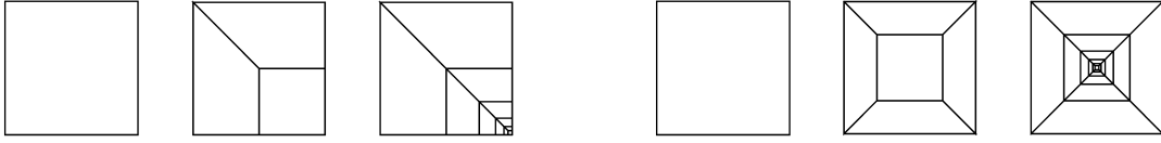
Fig. 5.3. To avoid hanging nodes, ultraSEM performs h -refinement in a conforming way. (Left) A square is successively refined into a corner by subdividing into three children per refinement level. (Right) A square is successively refined around a point by subdividing into five children per refinement level. General quadrilaterals are refined in similar ways.
