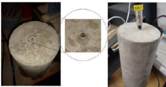
Figure 3. Thermal Conductivity test set-up
