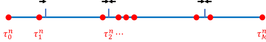
Figure 2: This figure illustrates an example of an admissible sequence; see Definition 9. For a fixed n , the red dots form the increasing sequence \{\tau_k^n\}_{k=0}^M . Note that the end points of the interval are included in the sequence, i.e., \tau_0^n = 0 and \tau_M^n = 1 . In view of Definition 9, as n \rightarrow \infty , the sequence \{\tau_k^n\}_{k=1}^{M-1} converges element-wise to three distinct points on the interior of the interval, shown with blue bars. Moreover, all limit points in (0, 1) have an even multiplicity except for one, which has a multiplicity of exactly one.
