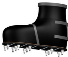
Figure 1: CAD design of sole morphing astronaut overboot.
