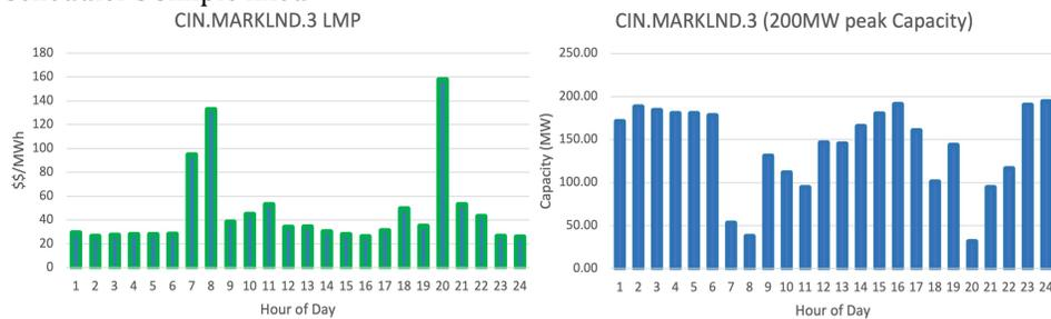
**Fig.4.** Power price (\$/MWh) (left) and resulting resource capacity for a 200 megawatt datacenter (right), using constant cost purchase approach. Exemplar 24-hour day from MISO January 9, 2018, CIN.Marklnd grid node.
