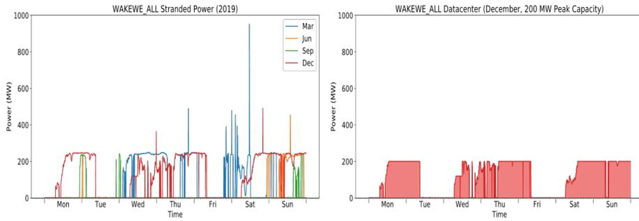
**Fig.6.** Stranded Power (curtailed and negative priced power) in 15-minute intervals for a node in the ERCOT power grid (left, each line is a different week), and the resulting resource capacity for a 200 megawatt datacenter for the week in December (right).
