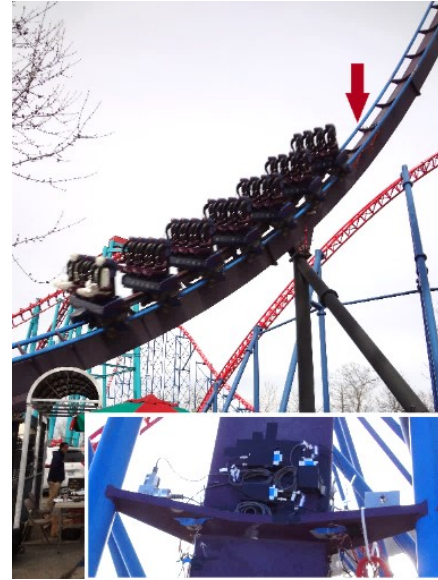
Fig. 2 Instrumented bracket location with close-up view of bracket and instrumentation.
