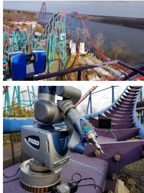
Fig. 7 Scanning of rollercoaster section. Top: 3D LiDAR Scanner. Bottom: CMM arm.
