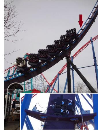
Figure 1 Instrumented bracket location. Close-up view of instrumentation.
