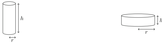
(a) This rigid body is inertially oblong if h^2 > 6r^2 . (b) This rigid body is inertially oblate if h^2 < 6r^2 .
