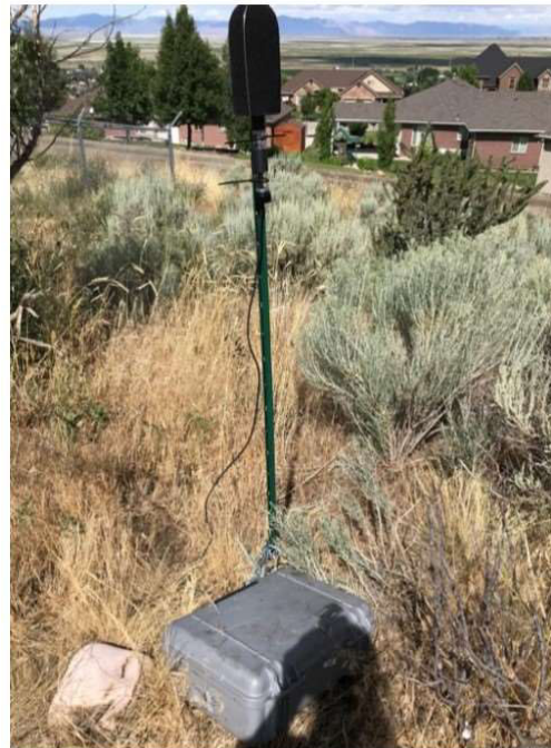
Figure 7. Data acquisition setup for collecting measurements of outdoor ambient sound.
