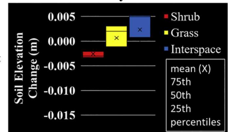
Fig. 7. Results obtained from using ground-based LiDAR to monitor rangeland soil fertility microsite types (SFMT) to characterize the source and sink dynamics of sediment and adsorbed nutrients at very high resolution and spatial accuracy. (A.) Example of mosaicked digital images acquired from the calibrated LiDAR-mounted camera during the LiDAR scans for one of the study plots in 2016, 2017, and 2018. (B.) Bare earth LiDAR point cloud colored by the machine learning SFMT classification and overlain by the vegetation points in each respective LiDAR point cloud for the example study plot. (C.) DODs derived from change detection of bare earth DEMs for 2016–2017 & 2017–2018 time series, respectively, from the example study plot. In the DODs, cool colors show locations of soil and adsorbed nutrient deposition and warm colors show locations of erosion caused by sediment transport associated with the disturbance of rangeland vegetation by fire and subsequent recovery of vegetation. Note that the same study plot is depicted in A, B and C but the vantage point differs (e.g., see the location of plot corners marked a and a' in each panel.). (D.) Soil surface elevation change (m) caused by erosion or deposition of soil determined from the DODs for the first- and second-year post-fire for all the burned monitoring plots. Note the shift in source and sink dynamics for sediment and adsorbed nutrients with post-fire recovery of the rangeland.
