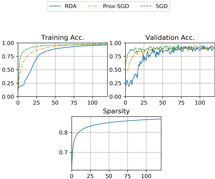
Fig. 1 An example of the first 120 epochs of loss and accuracy curves for different methods, and the sparsity curve of RDA on ResNet-18, CIFAR-10
