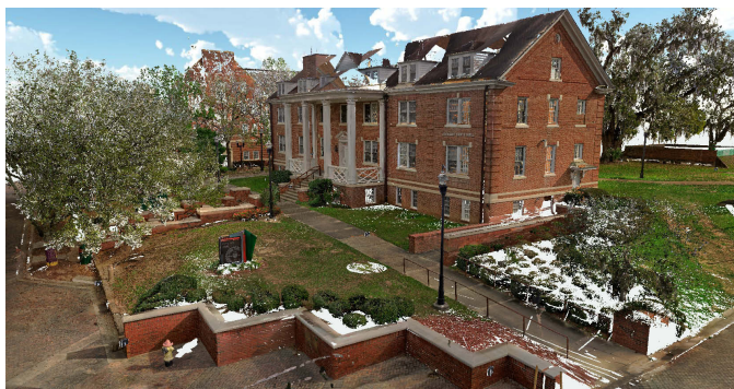
Fig. 6. 3D point cloud data from laser scanning done on FAMU campus.
