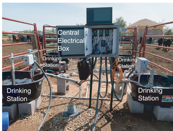
Figure 7. Setup at system test site with a central electrical box and four drinking stations.
