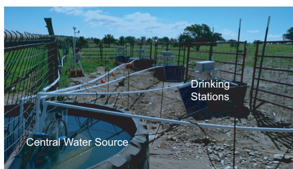
Figure 6. System setup at a remote testing site with drinking stations and a central water source.
