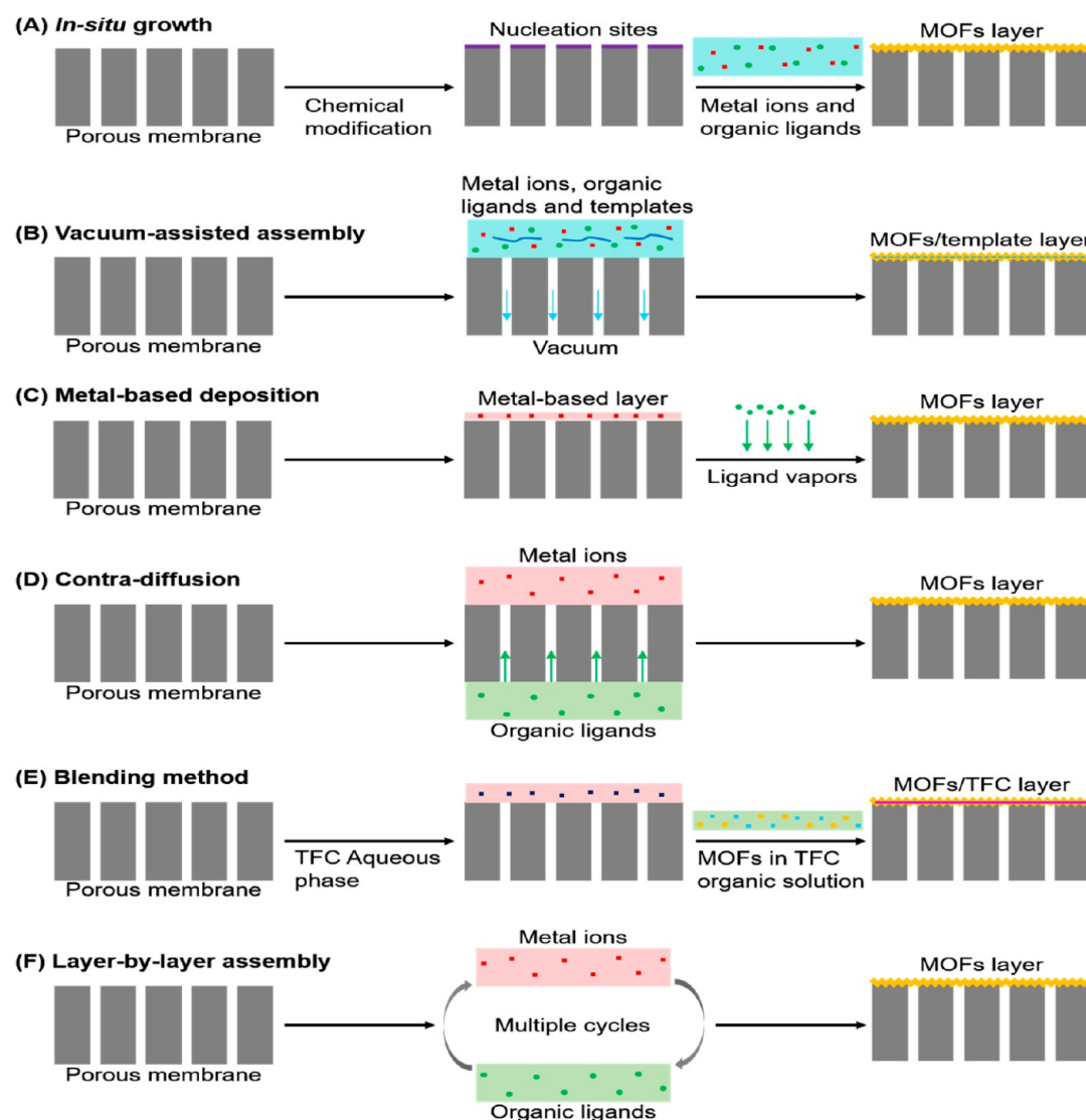
Figure 12. Schematics of fabrication strategies of ultrathin MOF-based membranes for organic solvent nanofiltration: (A) in situ growth, 264,268 (B) vacuum-assisted assembly, 265 (C) metal-based deposition, 19,267,274,275 (D) contra-diffusion, 162,276,277 (E) blending method, 49,55,66,70,71,109 and (F) layer-by-layer assembly. 266 Reproduced with permission from ref 261. Copyright 2019 Royal Society of Chemistry.
