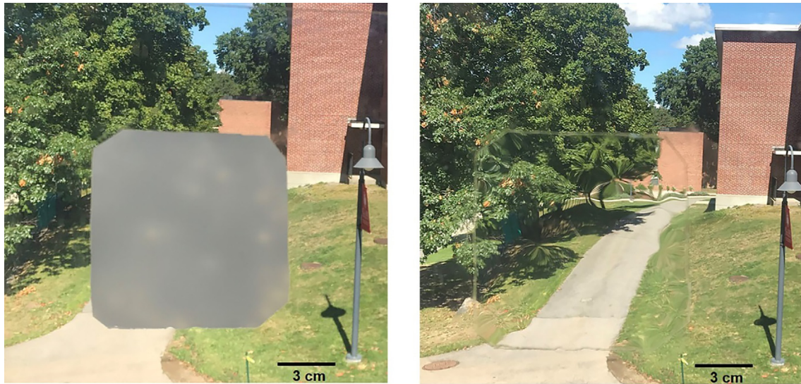
Fig. 1. the change of transparency in two phases. Left: cold, crystalline, and opaque. Right: hot, amorphous, transparent.
