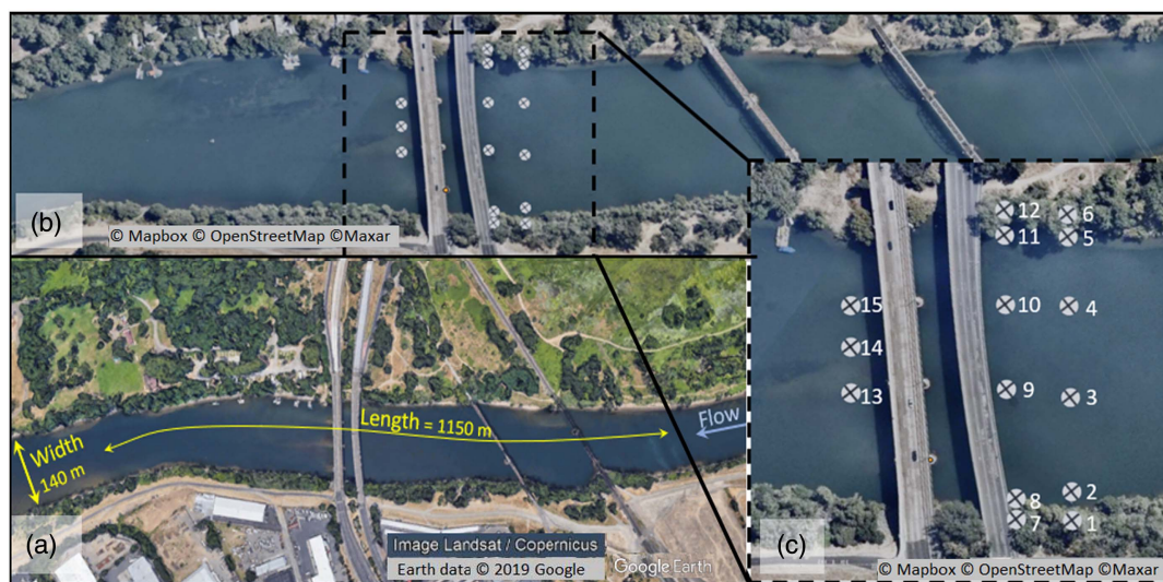
Fig. 5. American River indicating: (a) study area limits; (b) overview; and (c) zoomed-in area where computed velocity components and pressure were saved. The mean-flow depth at the site is \sim 12.2 m. [Map data for (a) from Google Earth, Earth data © 2019 Google, Image Landsat/Copernicus; map data for (b and c) from © Mapbox © OpenStreetMap © Maxar.]
