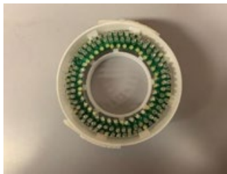
Figure 1: Printed light frame in ABS material with LEDs and plastic circuit board.
