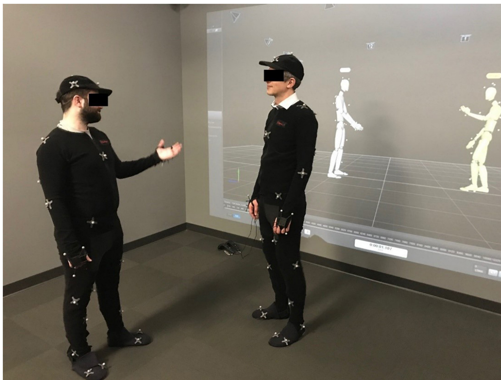
FIGURE 1 | Posed interaction showing the setup and the interface of the capture software as projection in the background (180° rotated).
