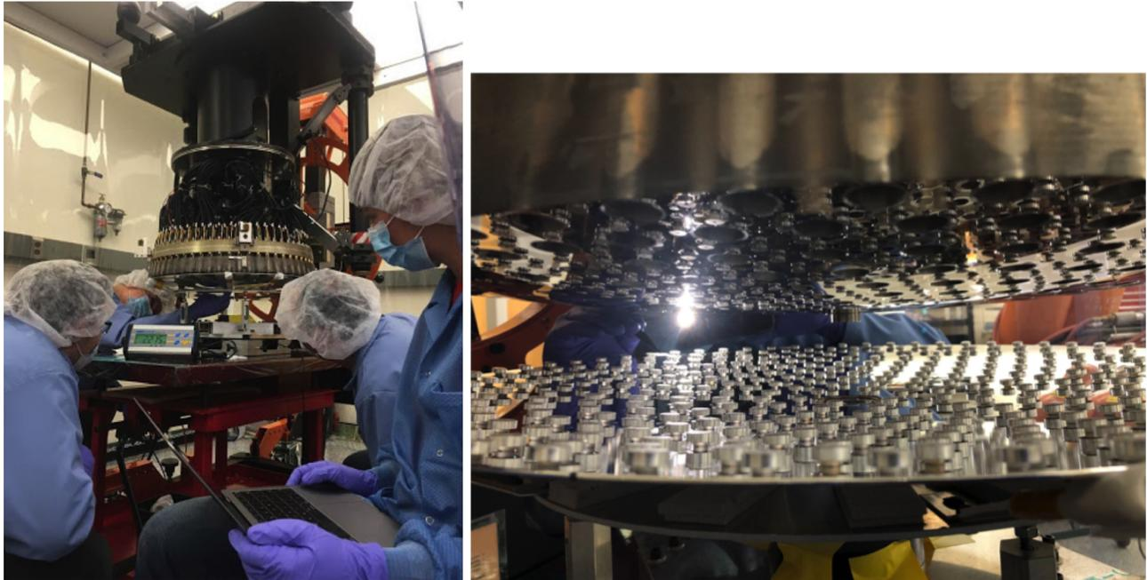
Figure 3 **Left:** Mounting the thin shell onto the reference body. **Right:** A look through the gap in the shell.
