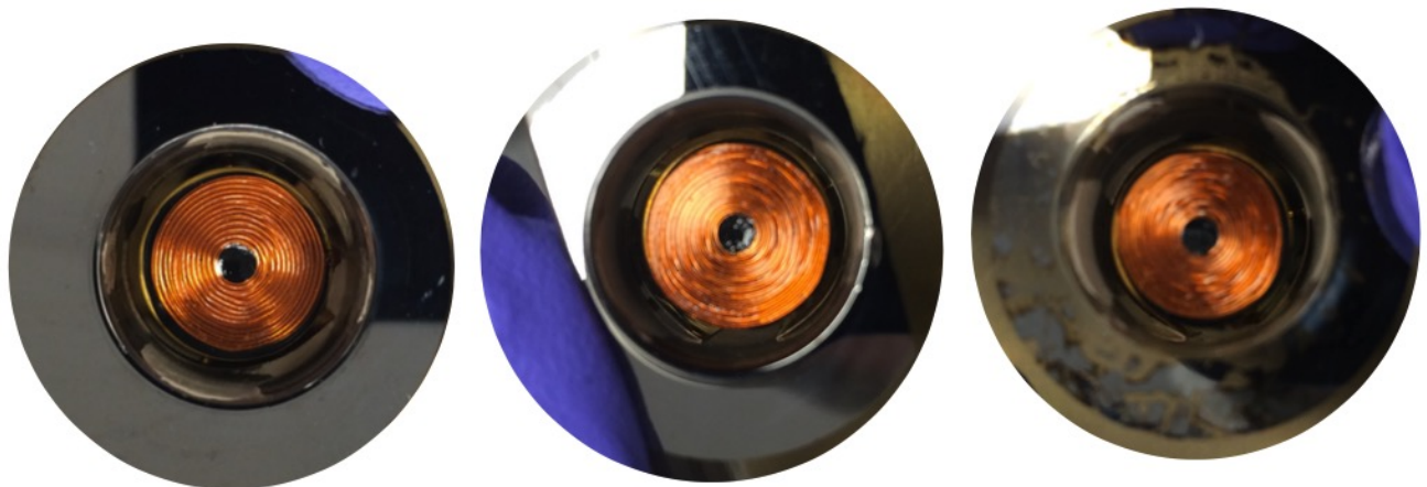
Figure 8 Armature inspection. Left to right: complete ring, edge ring, worst-scraped ring.
