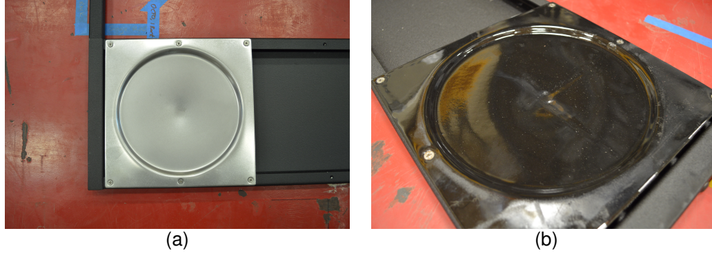
Figure 2.2: Rolling surfaces: (a) bare steel dish and (b) elastomeric lined dish.
