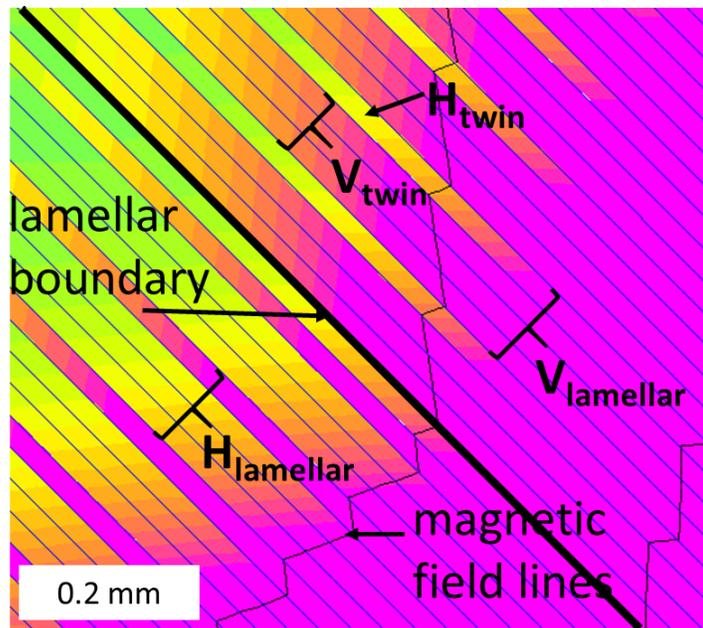
382 Fig. 11: Simulated flux schematic of the micropeened twin microstructure as defined by the ROI in Fig. 10.  $H_{\text{lamellar}}$
