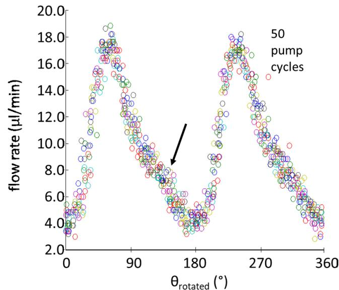
543 Fig. 15: Fifty MSM micropump cycles were superimposed, detailed, and adapted with permission from [43].  $\theta_{\text{rotated}}$
