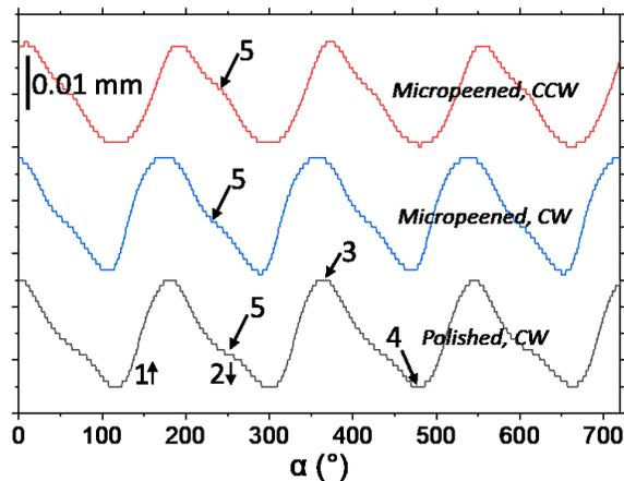
286 Fig. 6: Laser measurement at the center of the element as the magnetic field rotated. In black, the polished sample
