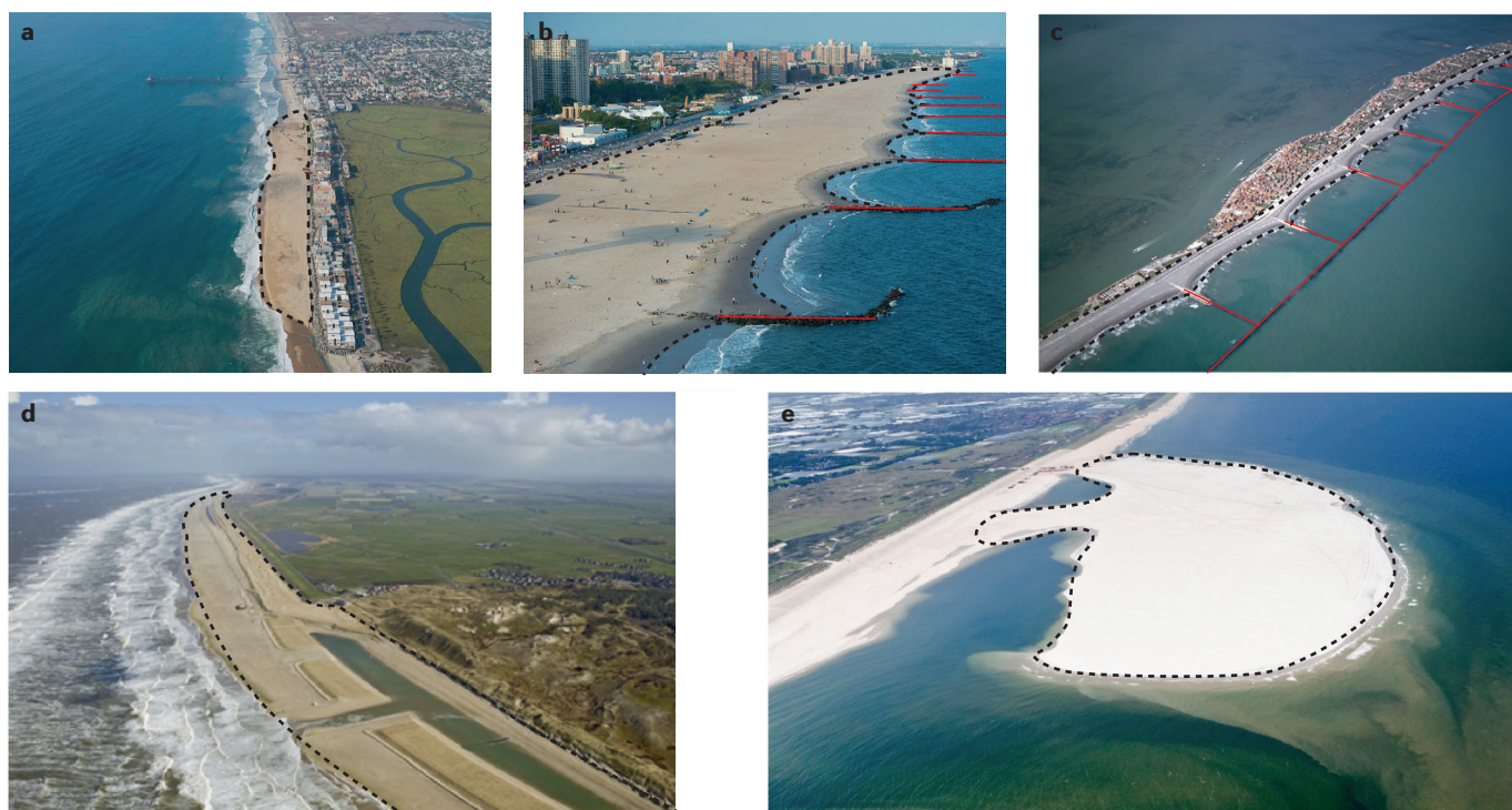
Fig. 1 | Beach nourishment projects. Nourishment sand bodies and additional hard structures indicated in black dashed and red lines respectively. a | Beach nourishment placement in progress, San Diego (USA). b | Beach nourishment with groyne field, Coney Island, New York (USA). c | Perched beach nourishment with groyne field and submerged sill, Pellestrina (Italy). d | Beach and dune nourishment with lagoon, Hondsbosse Dunes (the Netherlands). e | ‘Sand Engine’ mega nourishment intended to feed adjacent beaches with constructed lake and lagoon for additional types of recreational and ecological habitats, Kijkduin (the Netherlands). Part a adapted with permission from REF. 54 , Elsevier. Part b credit: Getty images/Bloomberg. Part c credit: Mauritius images GmbH/Alamy Stock Photo. Part d image courtesy of Royal Boskalis Westminster N.V. Part e image courtesy of Beeldbank Rijkswaterstaat/Joop van Houdt.
