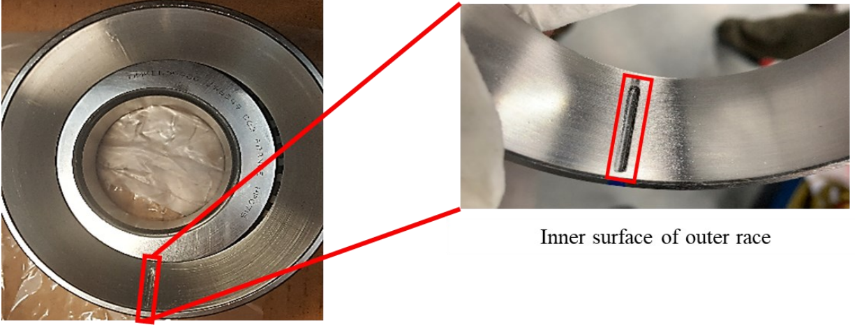
Figure 7. A single-point peck milling slot defect on the inner surface of the bearing outer race
