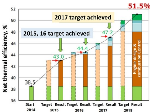
Fig. 3. Achieved engine net thermal efficiency of lean burn gasoline engine by the SIP program in Japan [2].
