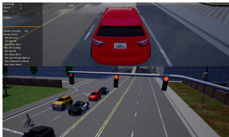
Figure 5: CARLA interfaced with DASC. The top pane displays the third-person view of a single vehicle while the bottom pane shows the view of multiple vehicles.
