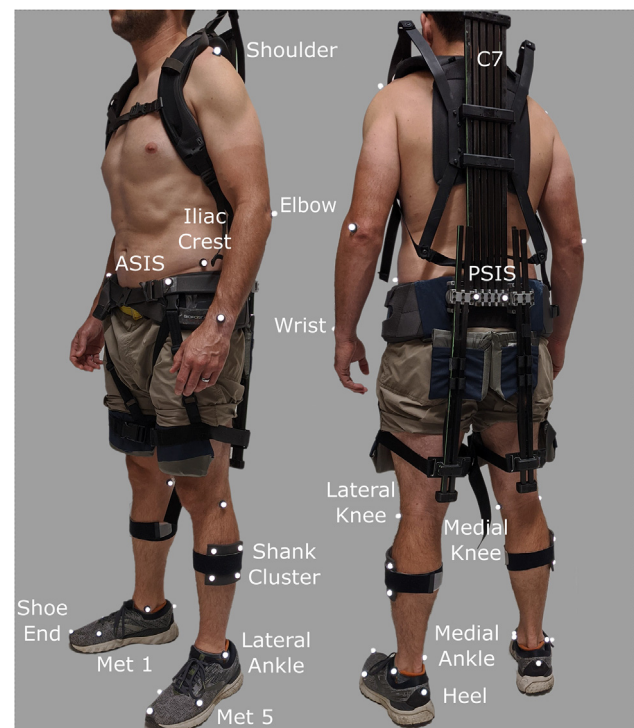
Fig. 1. Motion capture marker placement. The shoulder marker is placed on the acromion process. The elbow marker is placed on the lateral epicondyle of the humerus. ASIS and PSIS are the anterior and posterior superior iliac spine respectively. All markers are placed on both the left and right side of the subject.
