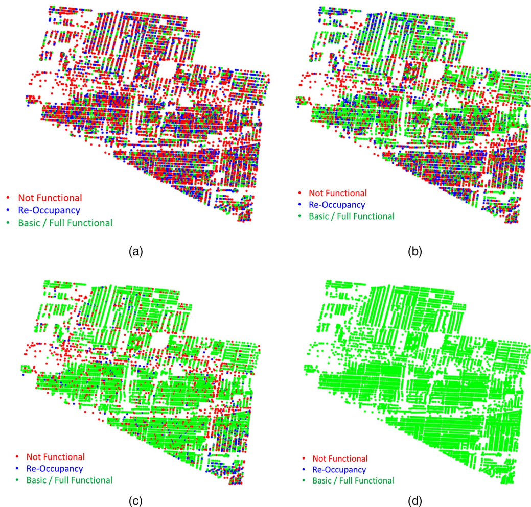
Fig. 12. Spatial distribution of the functionality of the buildings in the studied community for one arbitrary Monte Carlo simulation: (a) immediately after the earthquake; (b) after 30 weeks; (c) after 60 weeks; and (d) after 240 weeks.
