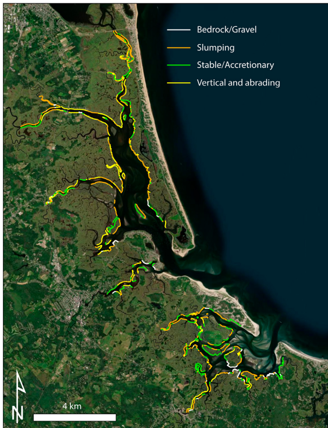
Fig. 3. Edge erosion map indicating mapped areas and their edge classification.
