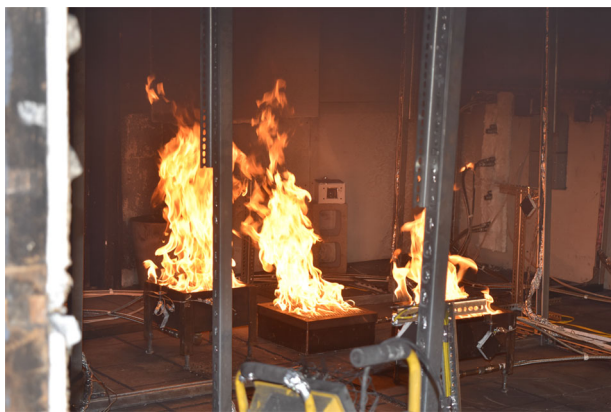
Figure 2. Photo of three burner fire evolution test captured through open door in the compartment during scoping tests. The HRR of burners 1, 2, and 3 were at roughly 70 kW, 100 kW, and 50 kW respectively. Flame heights remained well below the ceiling and minimal flame leaning was observed.
