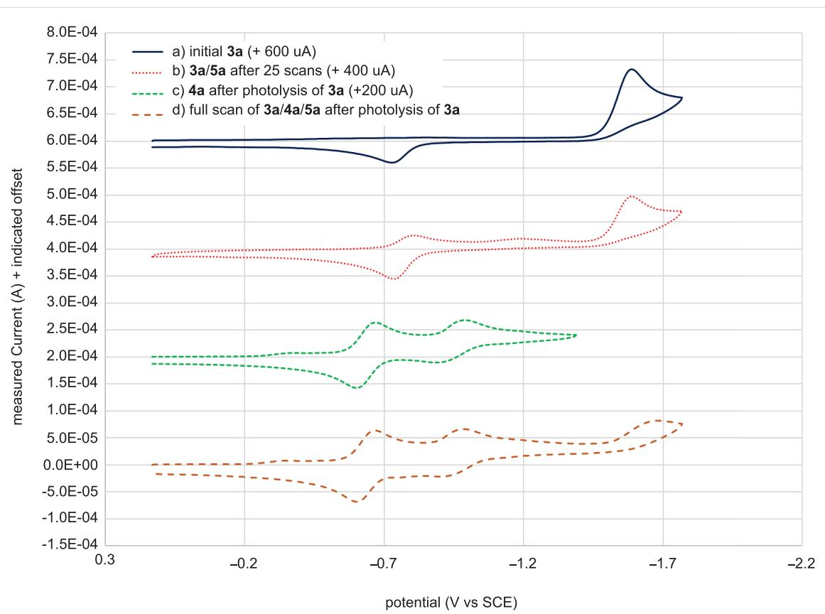
**Figure 4:** Cyclic voltammograms of a) **3a** before irradiation or electrolysis (solid blue), b) **3a** + **5a** after 25 scans (dotted red) showing the growth of the two eLW **5a** reduction peaks, c) **3a** after photolyzing but without reducing **3a** in the electrolysis (dashed green) which shows the two different reversible redox waves observed for pLW **4a**, and d) **3a** + **4a** + **5a** scanning the full potential window after the photolysis (dashed orange).
