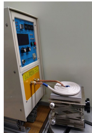
Figure 3. HT-15KW induction power supply with a small solenoid used in home ironwork process (left), pancake induction coil placed in the same power supply on top of the workpiece and ceramic mold (right).
