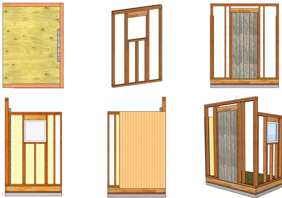
Fig. 1. Design exhibits of the wood frame.
