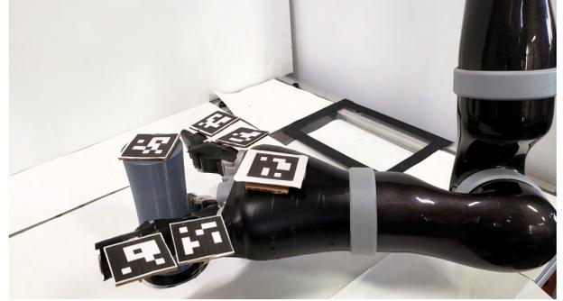
Fig. 4: Real world test setup. The ArUco markers were used to measure the finger, object and palm location and the box was used to tell if grasps were successful or not.
